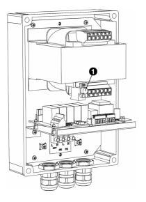
The control box is equipped with a fuse  ${\bf 0}.$
